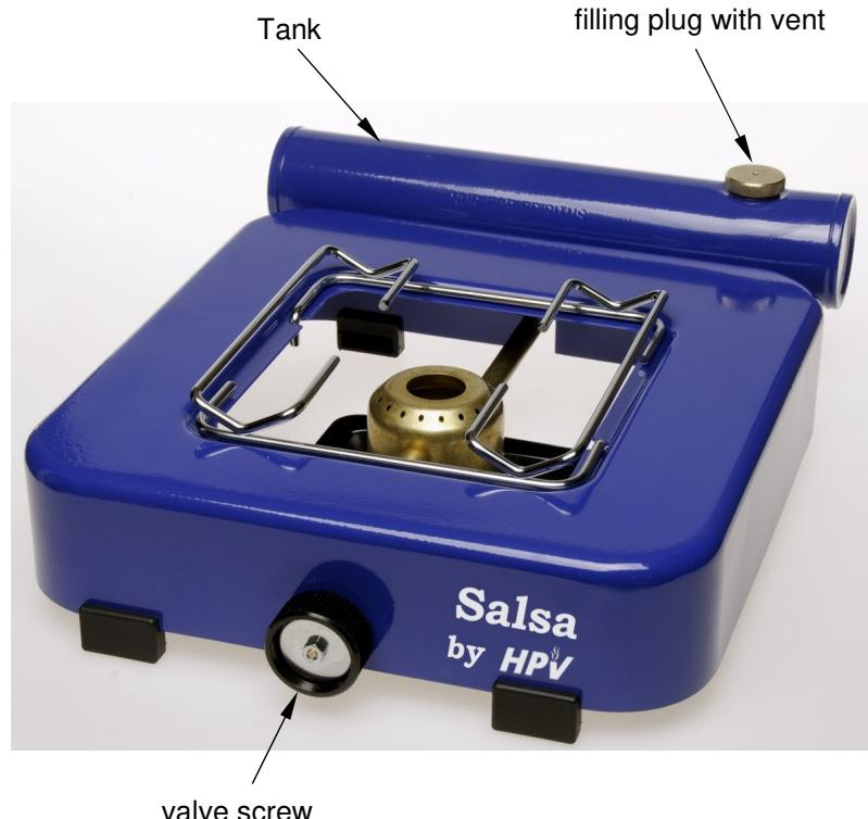
**Never top up spirit while the stove is burning or still hot. Always keep the vent in the filling plug of the tank open.**
