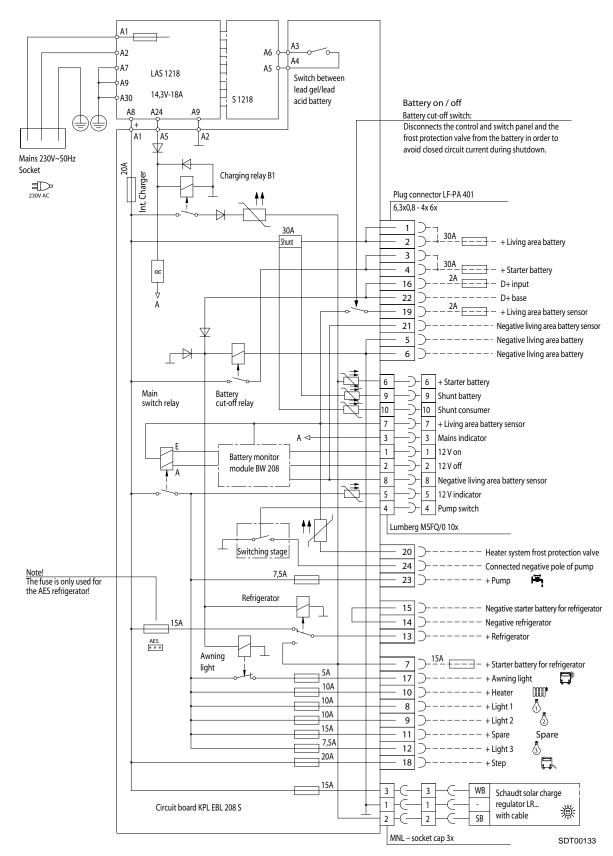
Fig. 2 Block diagram for Electrobloc EBL 208 S G
