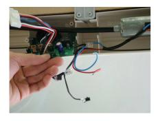
1.2.2 Disassemble the cables from the board, remove the old board, install the new board and connect the cables again.
