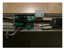
1.2.3 Remove the existing distribution board (with/without fuse) inside the interior frame and install the new distribution board with fuse.
